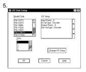
In the I/O Unit Setup screen's [Model Code] selection box, click on [FN-XY08TS] and click on [OK]. Control then returns to the Configure I/O screen.
