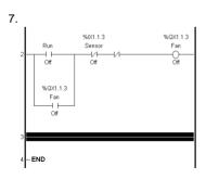
To insert a new rung below Rung 2, select Rung 2 and click on the  $\boxed{|+]}$  icon.
