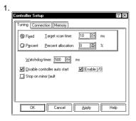
Settings for Using External I/O. In the Pro-Control Editor [Controller] menu, select [Setup] and the [Setup] dialog box will appear. Click on the [Tuning] tab. select (check)
