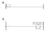
Click on the III icon to create a Normally-Open contact on Rung 3. (see diagram)
